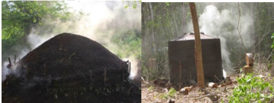
Figure 23. Different processes used to produce charcoal in the Yucatan Peninsula (traditional earth kiln, pit and metallic kilns).
